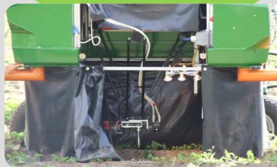
Transfer of weed positions, movement of manipulator to weed
